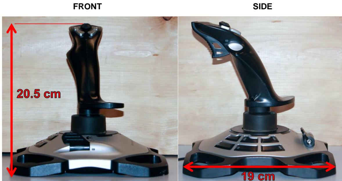
The RHC, shown above, had a range of rotational motion of about 20 degrees in each direction, with an approximately linear spring constant requiring the following forces at maximum displacement of the approximate center of grip (~10 cm from the pivot point, which is visually obscured by the rubber gasket):
