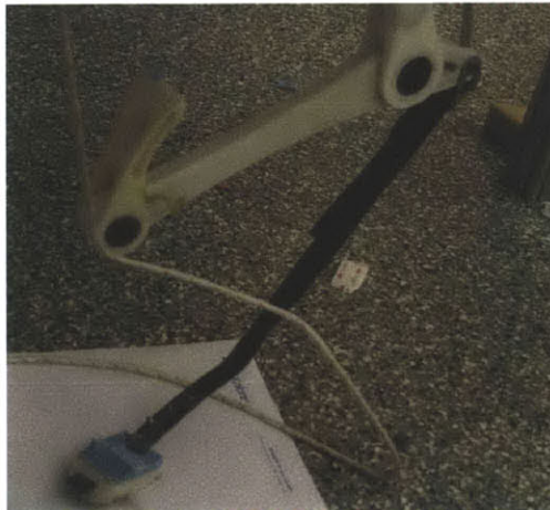
Figure 3-27: Kevlar tendon of the front leg, shown here during assembly of the foot pad. The tendon is connected to the tricep pin at the posterior end of the radius, from there it partially wraps the wrist joint and is embedded into the foot.
