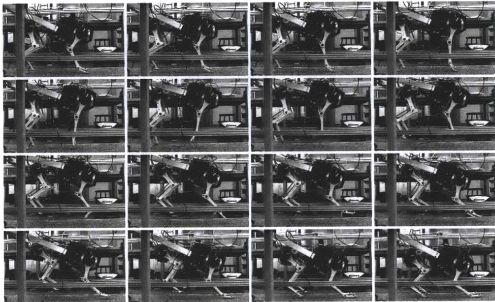
Figure 6-4: Vertical jumping of four legged robot.
