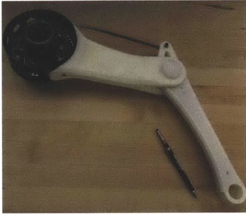
Figure 3-25: Front leg links assembled to the housing.
