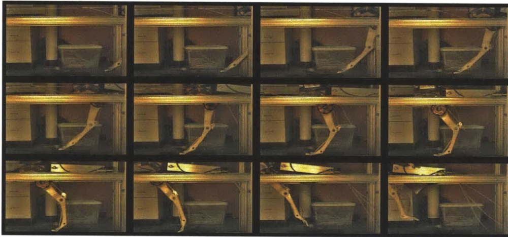
Figure 6-2: Still images from a high-speed video of single leg testing.
