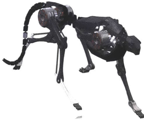
Figure 1-1: Conceptual model of quadrupedal robot showing four legs, compliant spine and tail.
