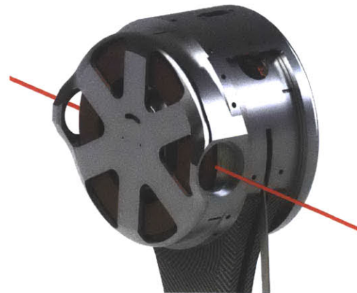
Figure 3-24: Ad/abduction mount on the shoulder unit permits rotation about an axis parallel to the spine shown here as a red line.
