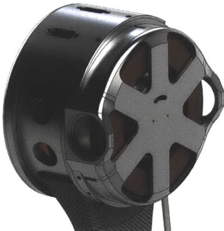
Figure 3-15: The shoulder unit of the front leg encloses both actuators, gearboxes and sensors.
