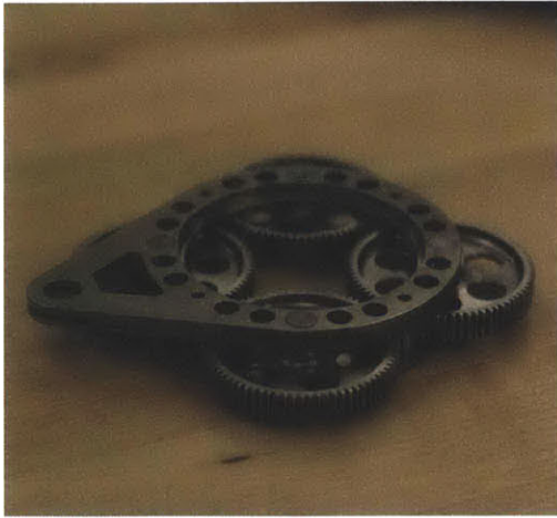
Figure 3-21: Assembled view of the planet carrier and planet gears.
