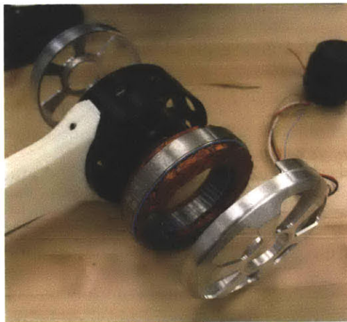
Figure 3-14: Allied Motion HT05001 torque motor, peak torque: 23.2 N · m, shown here with components of the front leg.
