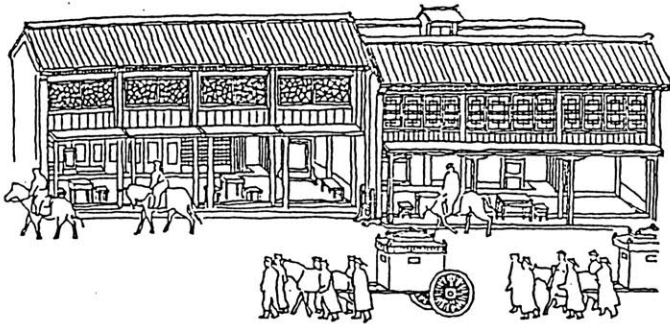
Fig. 3.33 Drawing showing movable partitions of store facades
