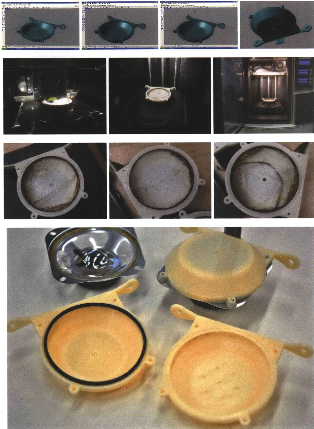
Figure D-5: 3D print of cavity and apertures for a multiaperture synthetic jet.
