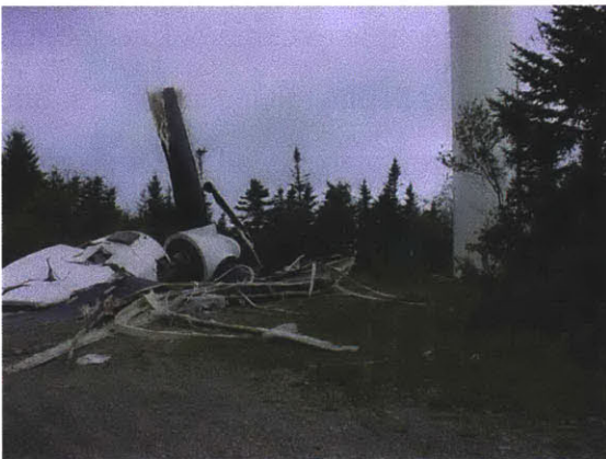
Figure F-1: “This turbine’s 28-ton nacelle and 3-blade rotor assembly crashed to the ground scattering debris several hundred feet from the structure. Approximately 20-gallons of heavy oil spilled from the unit when its fluid reservoirs were damaged. The 11-turbine Searsburg, [VT] facility was brought online in 1997 and [...] the Zond Z-P40-FS turbines had an expected lifespan of 30-years.” IWAG Press Release dated October 2008, retrieved April 2011.
