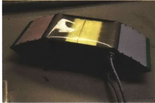
Figure 4-5: Underwater test object with moving surfaces.
