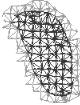
Figure 5-4: A thin slice through a tetrahedral mesh of a right thalamus. The dark tetrahedra are inside the thalamus. The lighter tetrahedra are outside the thalamus. During matching, the dark tetrahedra are attracted to region that are more likely to contain thalamus, the light tetrahedra are attracted to regions less likely to contain thalamus.
