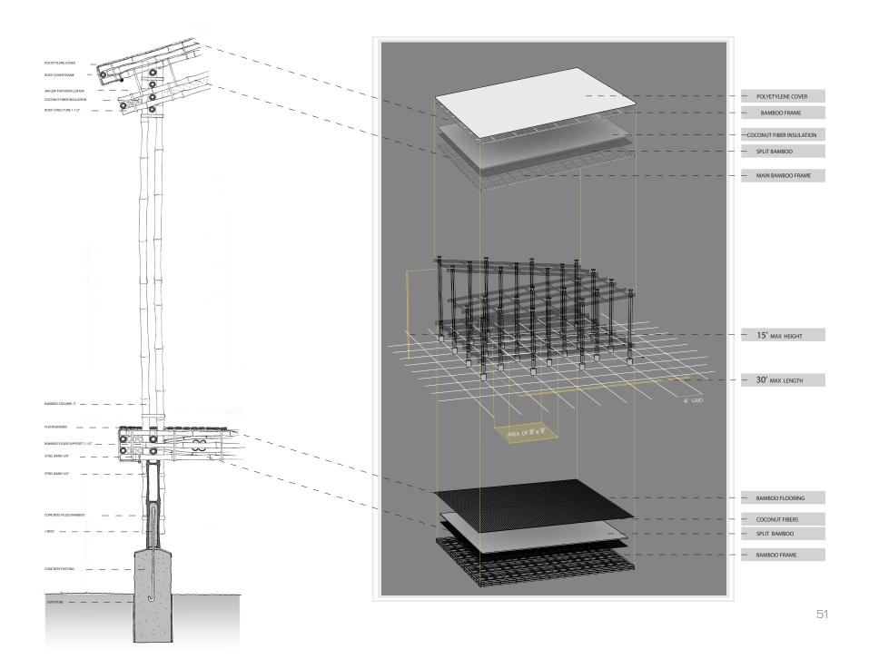
As most of the design, the column detail was also developed through construction. I built a full scale mock-up in order to test the proposed method. The structure allowed me to familiarize myself with the materials involved and the changes that need to be made when particular design details are difficult to fabricate.
