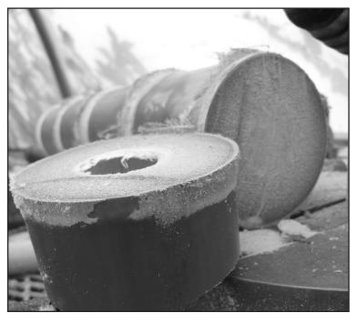
A very important part of researching bamboo was being introduced to some of its strongest species. The table to the right shows a list of some of the species that are most suitable for building construction and compares their compressive and tensile strength as calculated by Jules Janssen's formula in Working With Bamboo. We took samples from different parts of the bamboo poles and found their yield strength by finding their densities.
