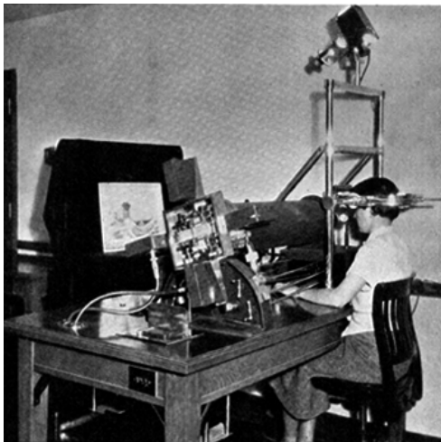
Figure 20: The photographic instrument that Buswell developed in order to measure eye movements of a human subject while examining a two dimensional picture. Here we see a subject seated at a laboratory bench with head stabilized. The photographic apparatus dominates the space of the table (seen to the left of the subject). The image is seen with a black background in the left of the image. The image being shown appears to be a reproduction of Katsushika Hokusai's color woodcut The Great Wave off Kanagawa , c. 1829-1832. Reproduced from Guy T. Buswell, How People Look at Pictures , plate V.
