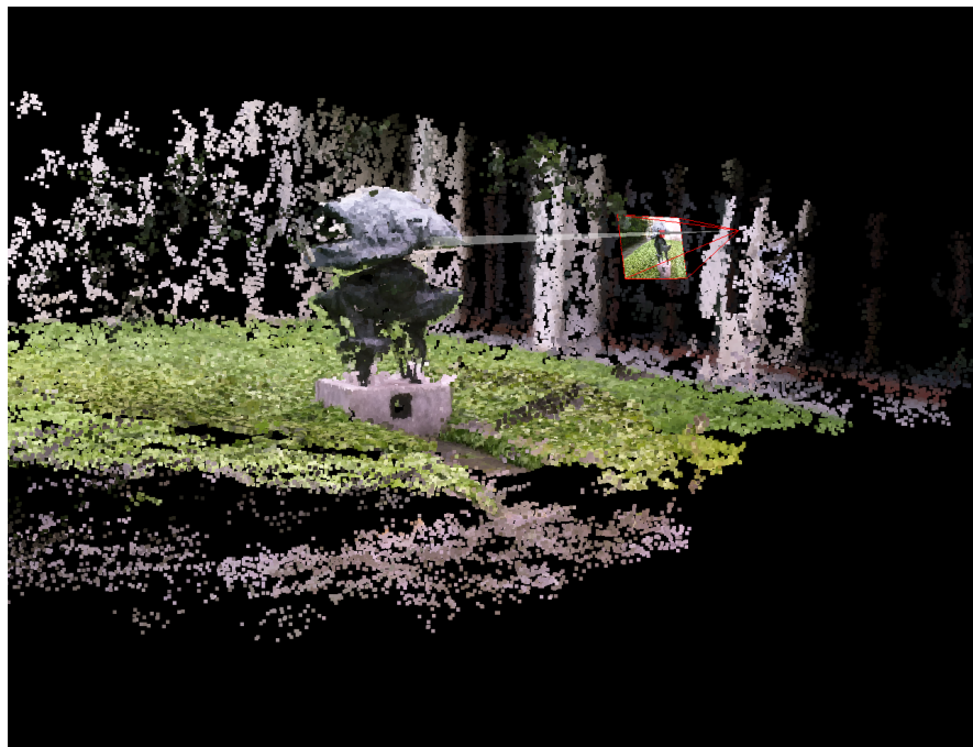
Figure 77: The same frame as the previous figure, now observed from a simulated third person perspective. The red pyramid represents the projection matrix corresponding to that image and the subject's pose in the world at that instant in time. The space constructed using SfM is shown here as a dense point cloud. The white cone describes the subject's volume of visual attention. This cone intersects with the three dimensional points, revealing the relationship between the subject's gaze and the world.
