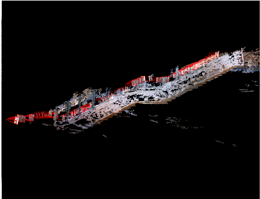
Figure 82: The subject walked up a flight of stairs from the second to the third floor of the Stata center at MIT. This is the subject's first encounter with this space. The red pyramids are the pose of the subject in the space. This capture lasted 30 seconds.
