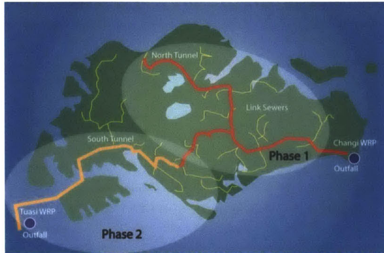
Figure 11 – DTSS pipeline layout (Loganathan 2008)
