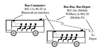
Fig. 2. Air interfaces for bus-commuter, bus-bus, and bus-depot communication.
