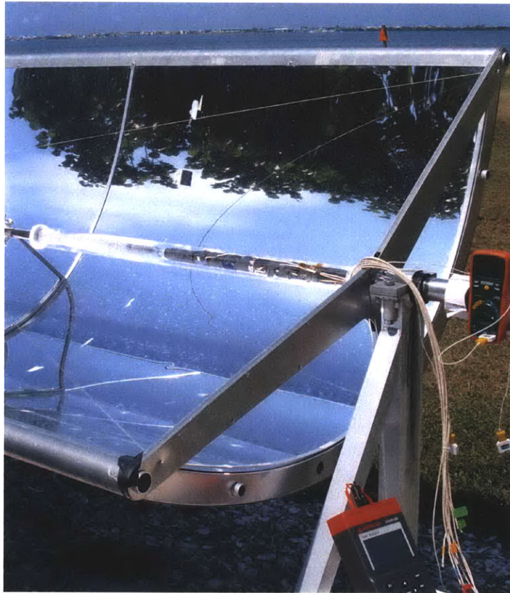
Figure 6-15: Experimental CPV absorber test section in the thermal loop of a SopoNova collector at Eckerd College
