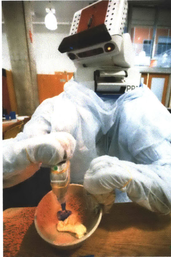
Figure 1-1: The PR2 in the protective garment. The garment mitigates the risk of spills and splashes during the cooking process.
