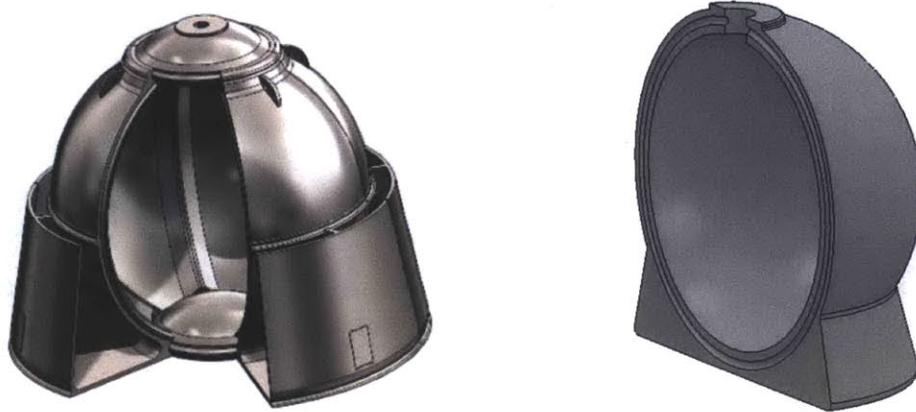
Figure 20 Multiple-stave sphere (on the left) compared to hemisphere design (on the right) (credit Alex Slocum)
