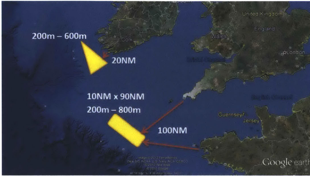
Figure 53 Western Europe has two possible deployment sites a total of 3086km 2 and 20 to 100NM away from shore
