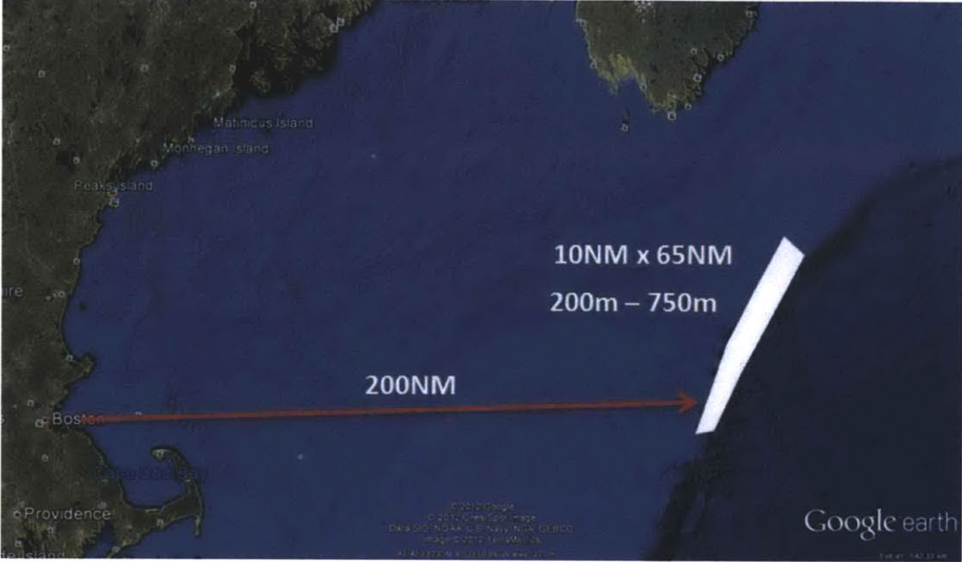
Figure 44 Gulf of Maine ORES deployment site. Total surface area available for ORES deployment is 2,230km 2
