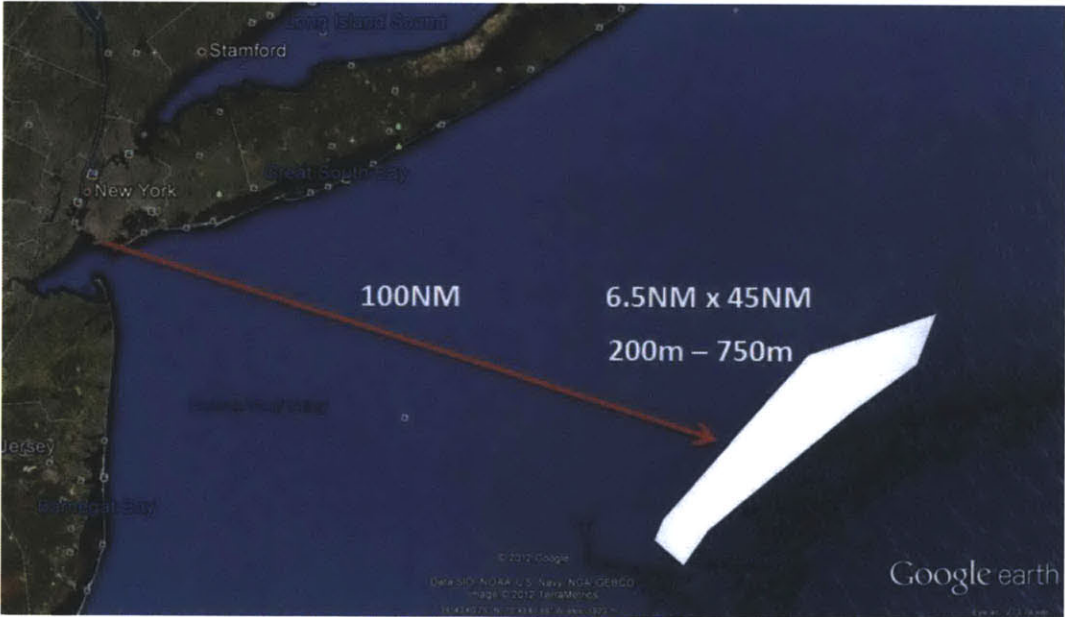
Figure 45 New York and New Jersey ORES deployment site. Total surface area in 200-750m depths range is 1,000km 2
