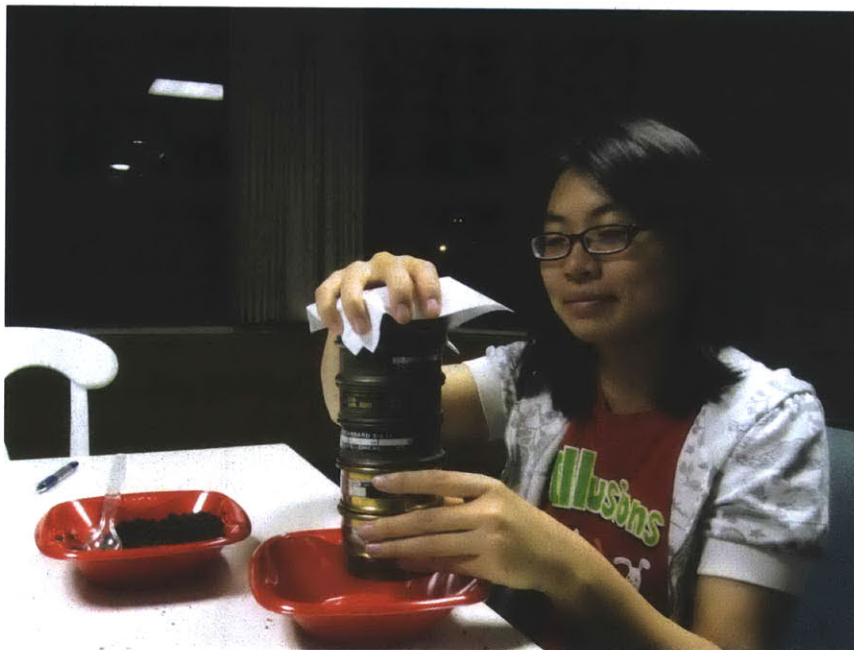
Figure 6.17: Manually agitating the stacked sieves to induce separation of the soil sample by particle size.
