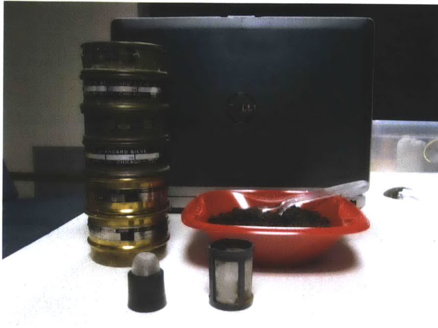
Figure 6.16: The experimental set-up of sieve analysis in order to determine the particulate matter that will pass through the filters of the PDIK systems.
