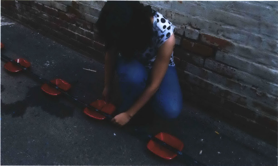
Figure 6.5: Adjusting the emitters such that the water flow is directed into the plastic bowls. Photo: Lisa Johnson (2012)
