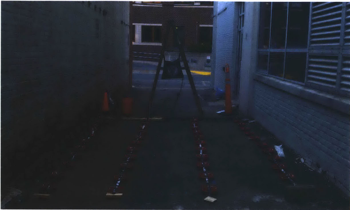
Figure 6.2: The experimental set-up of testing emitter flow rate performance for the IDE drip kit. Photo: Lisa Johnson (2012)
