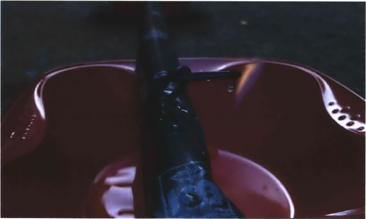
Figure 6.6: An emitter producing droplets into the plastic bowl. Photo: Lisa Johnson (2012)
