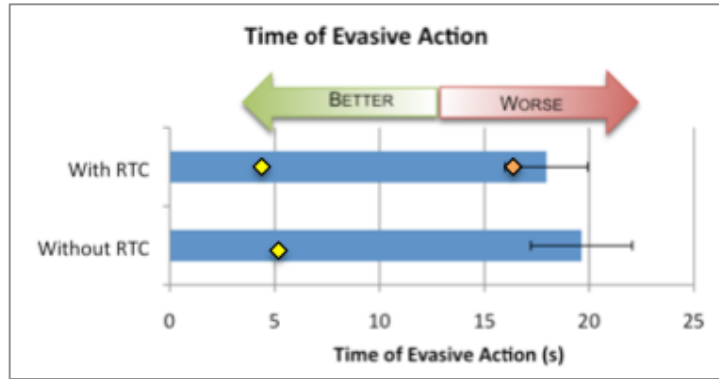
Figure 6-18. Time of Evasive Action for Vertical High Closure Rate Conflict in the Display System
