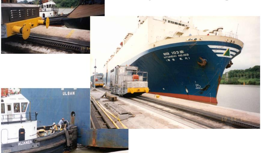
Locomotives hold the ship straight – the ship provides the power
