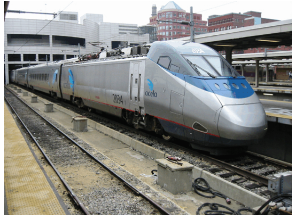
The cement stumps between the tracks are some of the foundations for the future air-rights developments.
