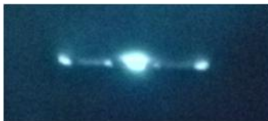
Figure 6- 17: Image taken by InGaAs camera. Later investigation shows this image is seen at the laser/waveguide coupling facet, as shown in Figure 6- 18.
