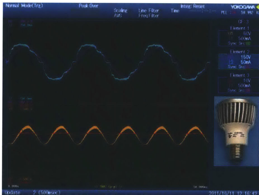
Figure 1-1: 6W, 3 LED input output voltage/current waveform.
