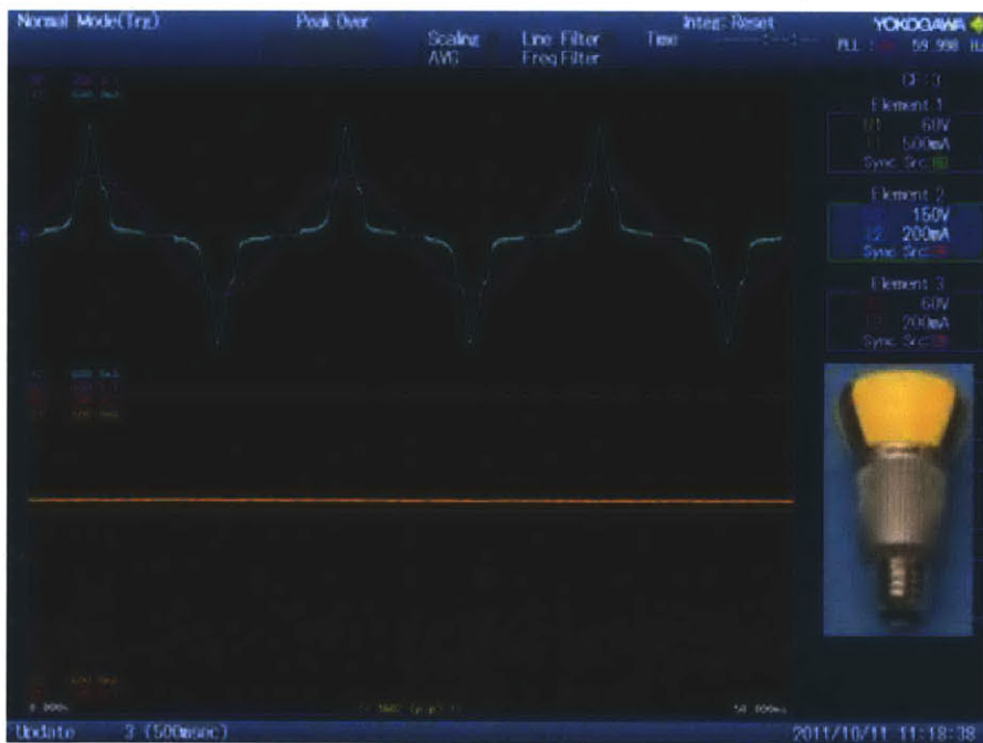
Figure 1-3: 12.5W, 18 LED input output voltage/current waveform.
