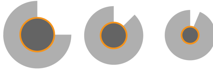
Figure 4-2: The light gray area represents the table surface, wrapped around poles of various sizes. In each of the three images, the gray surface is the same area, wrapped around various pole diameters.
