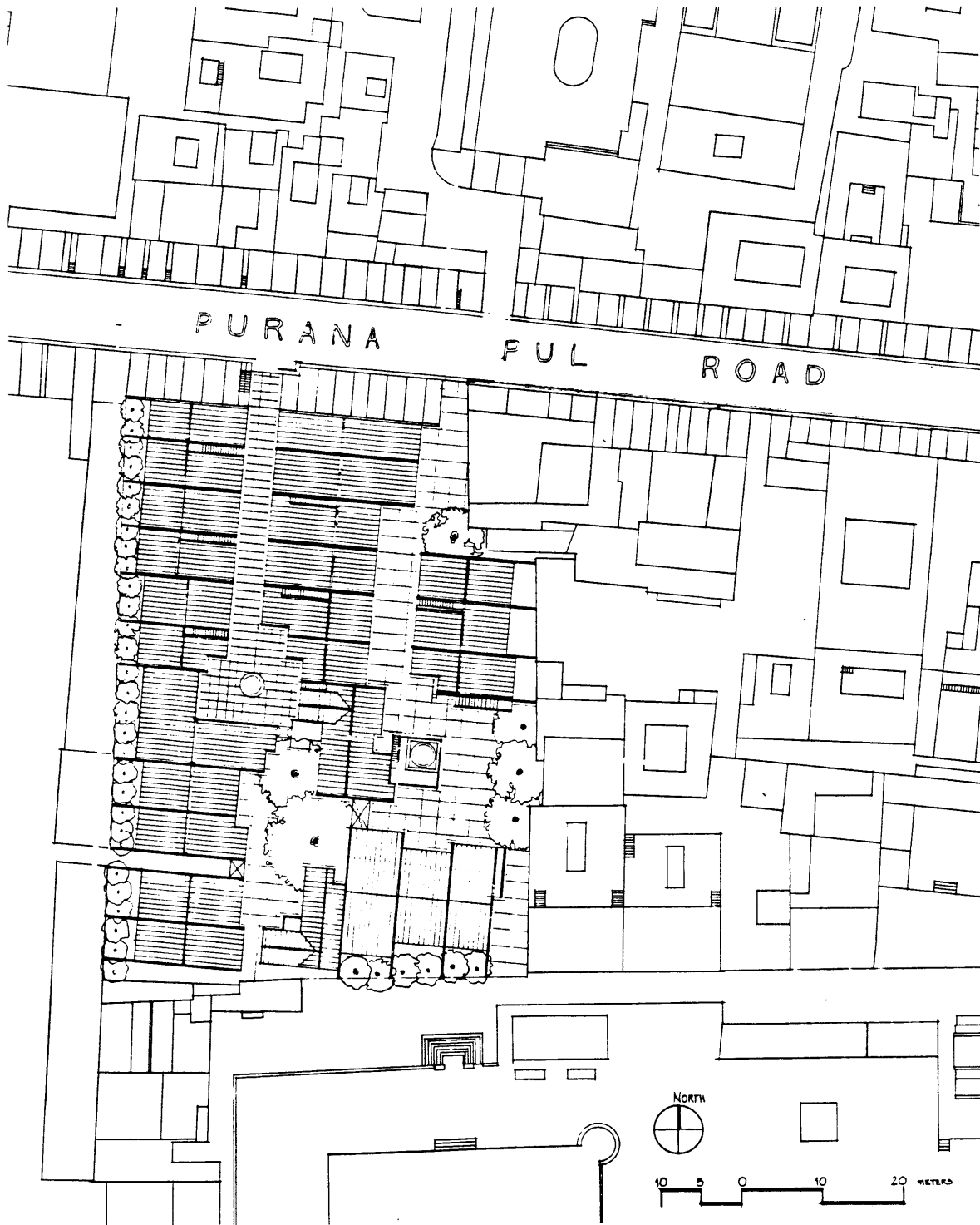
A proposal for two phases of development. The first is organized around arcade and shops at ground level with housing for the hutment dwellers up to three storeys. Second phase organized around courtyards -- larger, lower houses for middle and higher income groups.
