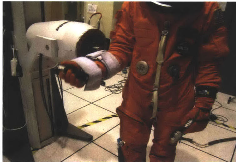
Figure 2.3 Primus RS™ collecting unpressurized ACES elbow torque data [Matty & Aitchison, 2009]
