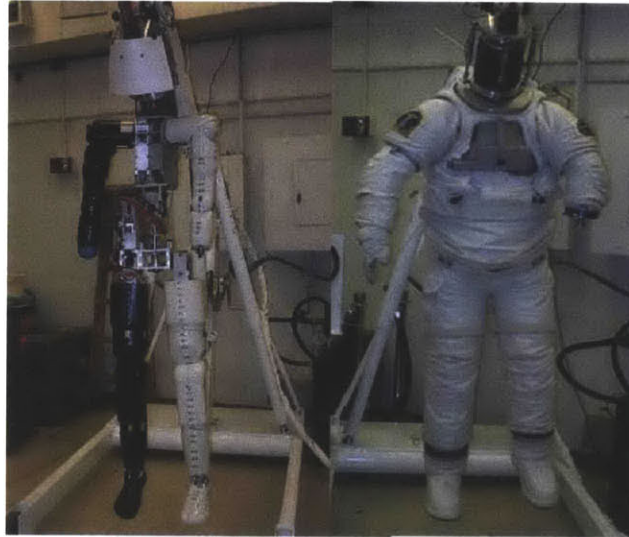
Figure 2.5 (a) Robot Space Suit Tester (RSST), (b) RSST with EMU installed [Schmidt et al., 2001]
