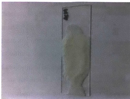
Figure 3.2.4: Film-casting from unclear solution as represented in Figure 3.2.3.
