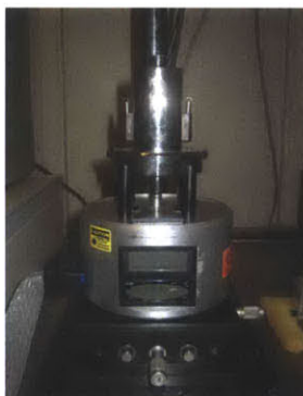
Figure 3.2 NanoScope IIIa Multimode AFM. (A) Piezo connected to the equipment controller. (B) Microscope head and cantilever holders. (C) Manufacturer schematic of the inner workings of the microscope head with a cantilever holder.
