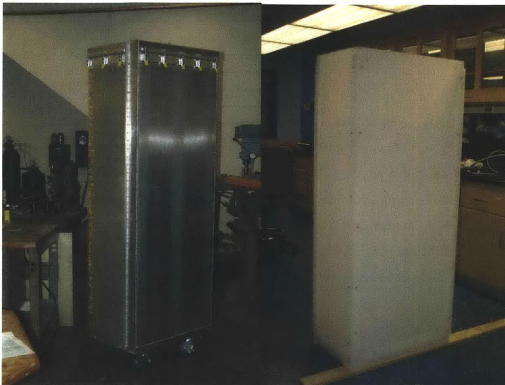
Figure 5-1. Aluminum body of the detector (left) and polypropylene insert (right).
