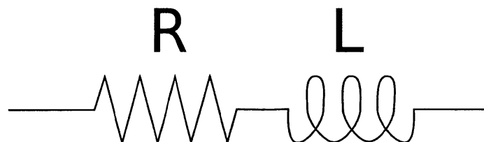
Figure 5-1: Simplified equivalent circuit for an electromagnet in the BBGS: a resistor and inductor in series.
