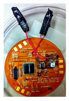
Figure 4.14: The populated CPCA (minus the jumpers) is shown. The two large components are  $220\mu$ F capacitors for the input of the voltage regulation stage.
