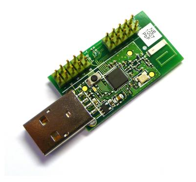
Figure 4.7: The Chipcon CC1111 board and debugger were used to program the front-end and ADC chip [49].
