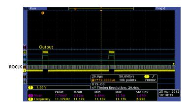
Figure 4.17: The output DATAVALID is approximately a 20% duty-cycled waveform. The ROCLK signal is also shown.
