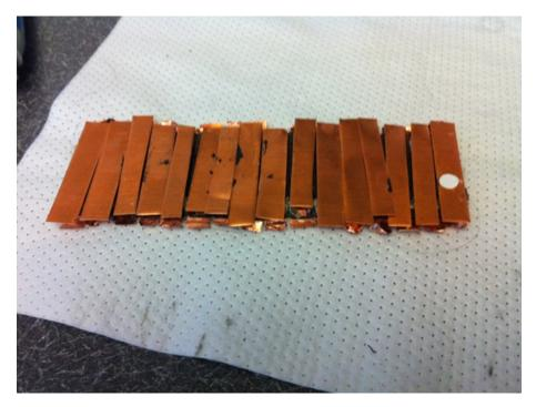
Figure 3.11: Upon thermally connecting the cold side copper strips with the ceramic, the flex TEG is ready for curing of the TIM (the white sticker was used to hold a thermocouple for thermal measurements).
