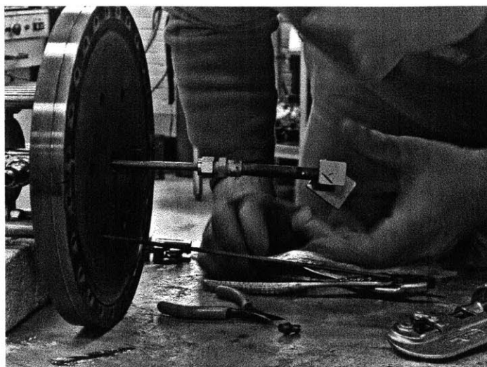
FIGURE 13. The samples being adjusted on the titanium rod. (The polished surface reflects the wood table, giving it a gold appearance in this photograph.) Note that the titanium rod was attached to the furnace lid with the same molybdenum wire, which was an ideal attachment wire in this experiment due to its strength, flexibility, and temperature resistance. The entire holder can be moved up and down. Also note the in-furnace thermocouple, which protrudes beneath the samples.
