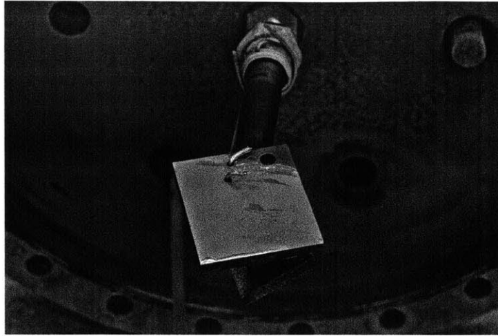
FIGURE 24. The F91 sample, after 30 hours of LBE exposure in a pure H_2 environment at 715^\circ C . Note that the vapor film on the inside of the lid is a grayish-blue color, instead of the yellowish film observed after the second test run, indicating that oxygen contamination was not an issue in this experiment.
