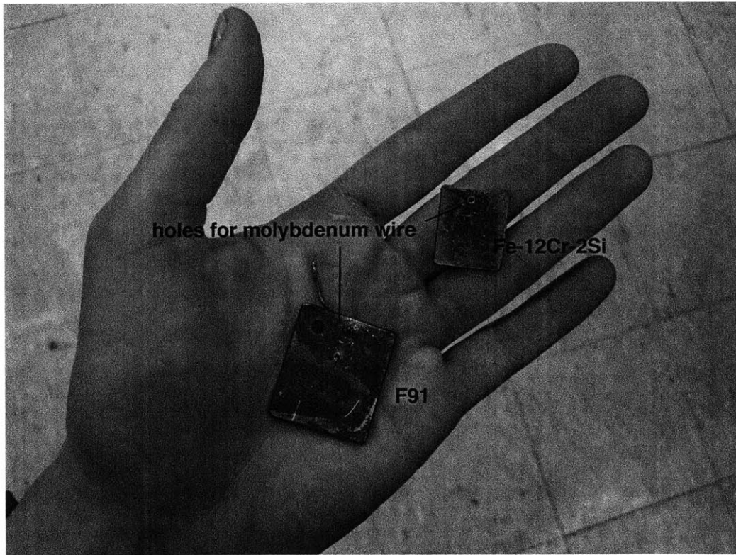
FIGURE 11. An exposed sample of F91 (bottom) is shown with an exposed sample of Fe-12Cr-2Si post-exposure. A thick, black oxide film has developed on their surfaces due to oxygen contamination during the experiment.
