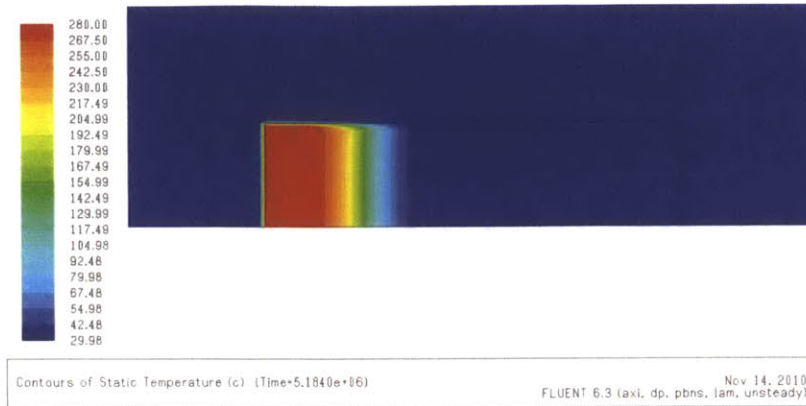
Fig.3-7 Transient Temperature Contour During a Charging Process: Case No.1, Length=1000m, Radius=250m: Time= 60 Days
