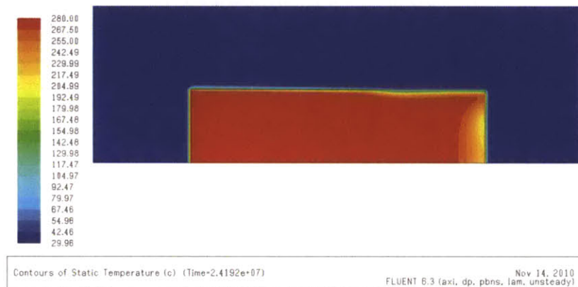
Fig.3-11 Transient Temperature Contour During a Charging Process: Case No.1: Length=1000m, Radius=250m: Time=280Days
