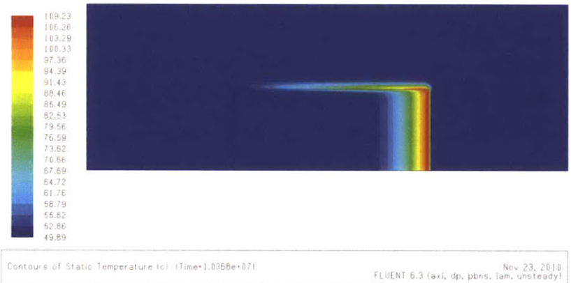
Fig.3-16 Transient Temperature Contour During a Charging Process: Case No.1: Length=300m, Radius=125m: Time=120Days
