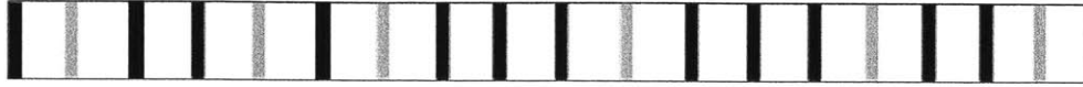
Figure 5-2: Example of lossy collection, where packets are randomly dropped with uniform probability. The black lines represent successfully transmitted packets, the gray lines represent lost packets.
