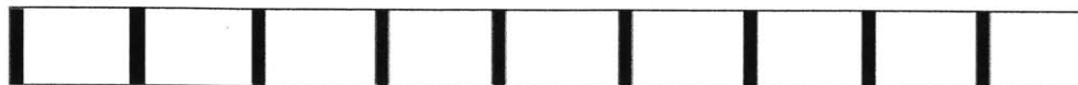
Figure 5-4: Example of downsampled collection, where the frequency of packet transmissions is decreased; no packets are dropped. The black lines represent successfully transmitted packets.
