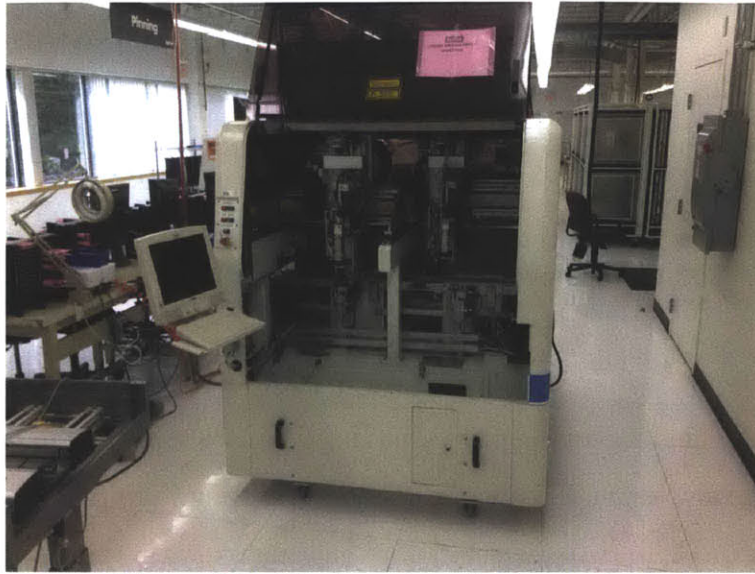
Figure 2-5: Dual-gantry pinning system
