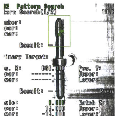
Figure 7-6: A successful pattern match for a pin in the opposite orientation. This pin is supposed to fail the pattern match test. The pattern match tool was not used in the application after obtaining such results on a repeated basis
