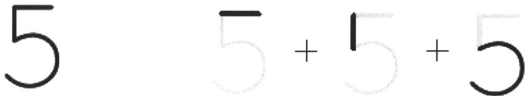
Figure 4-2: Structural features for the number 5, a horizontal and vertical line, and a curve [28]
