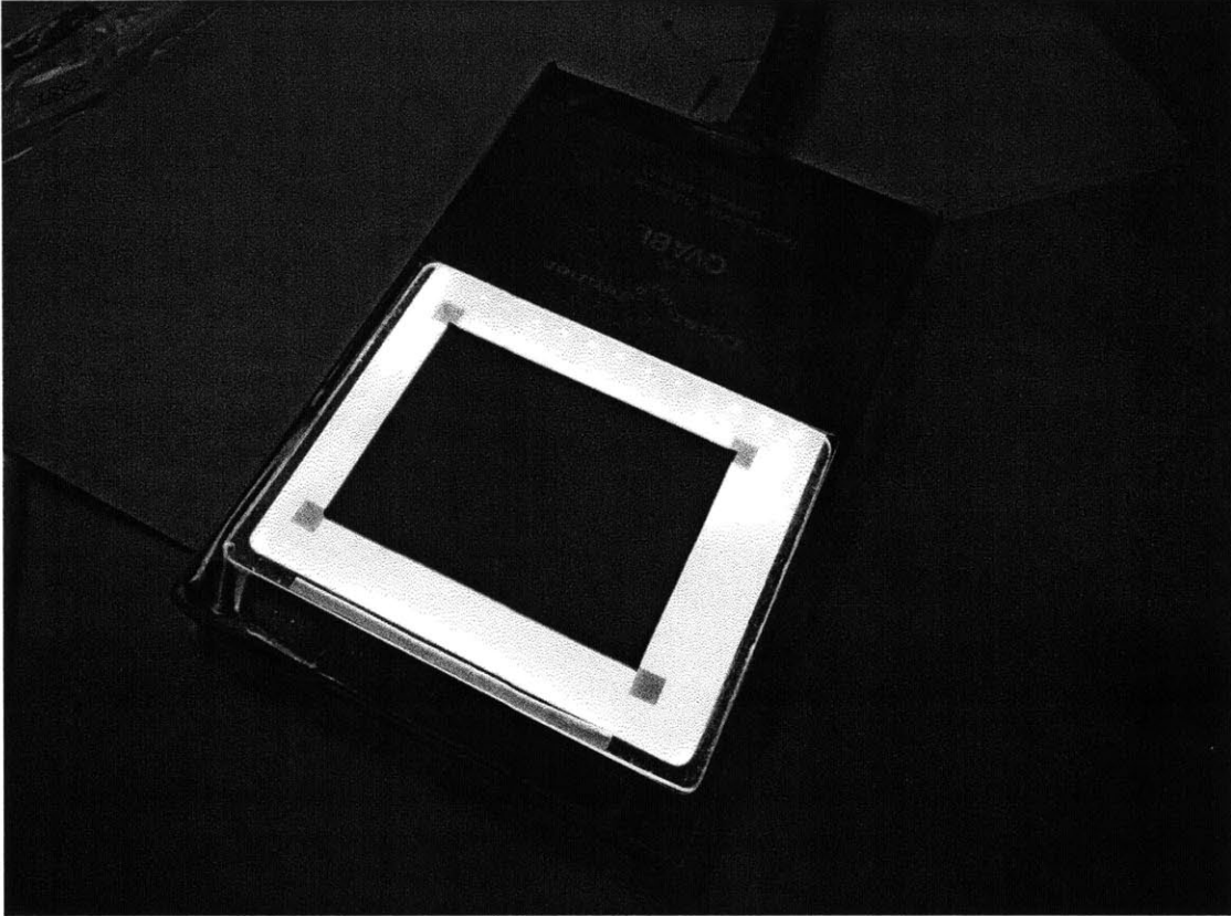
Figure 3.5: The backlight used in the manufacturing floor. The metal blocks the light and looks black under a microscope.
