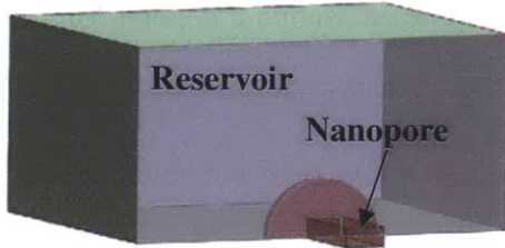
Figure 4.19 Environment for DNA transport around nanopore entry is approximated as spherically symmetric.
