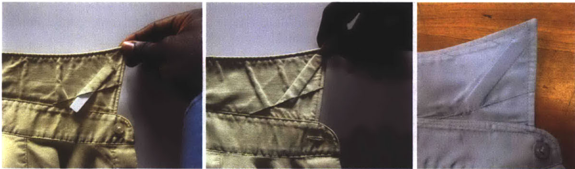
Figure 6-11. RFID tags inserted into collar stay slot.
