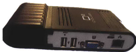
Figure 6-4. D2Plug ports (Source: Globalscale Technologies, Inc.).
