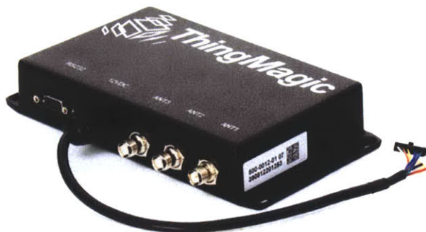
Figure 6-1. ThingMagic RFID Vega reader (Source: ThingMagic).
