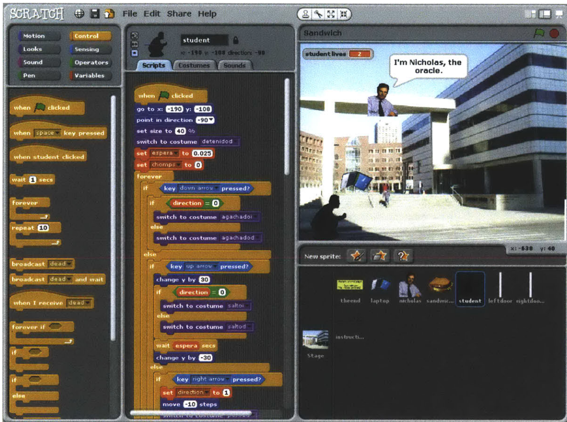
Figure 1-3: Scratch programming environment (version 1.4). The leftmost column represents an inventory of possible “programming blocks” which are assembled into program code in the center column. The area in the top right represents the project as it will be displayed to a user interacting with the finished product. The bottom right column shows the available sprites which are controlled by the code.
