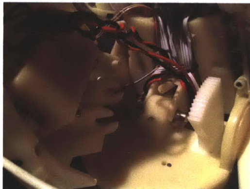
Figure 3-11: Waist bend mechanism and shaft clips for waist
