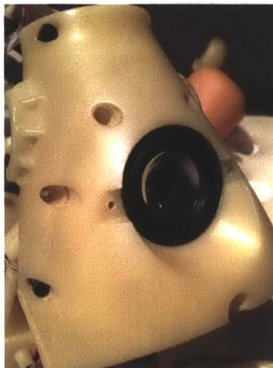
Figure 3-14: Speaker cavity in chest plate with speaker
