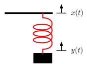
The mass is M = 1 kg and the spring constant is K = 1 N/m. Assume that the spring obeys Hooke's law and that the reference positions are defined so that if the input x(t) is equal to zero, then the resting position of y(t) is also zero.
