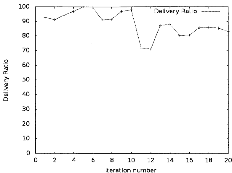
Figure 2-2: Delivery Ratio across 20 iterations for 2 nodes pinged each other
