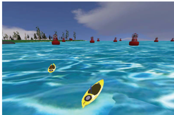
Fig. 2. Two ASCs performing CSLAM in a simulator developed in-house for testing and validation of algorithms before actual field trials.
