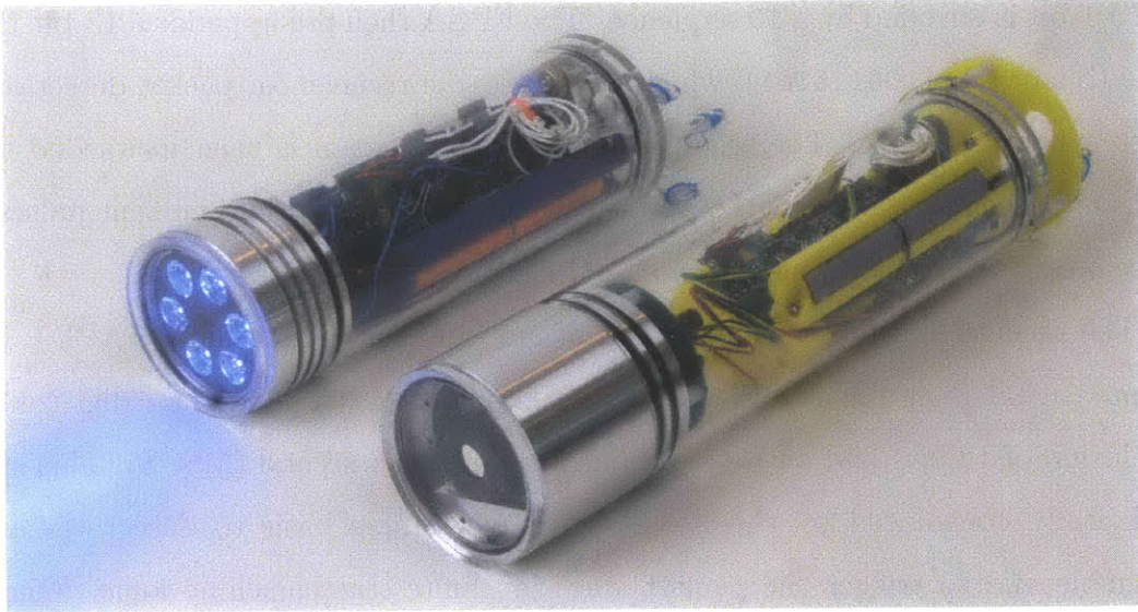
Figure 3-7: AquaOptical I modems. The transmitter is on the left and the receiver is on the right.
