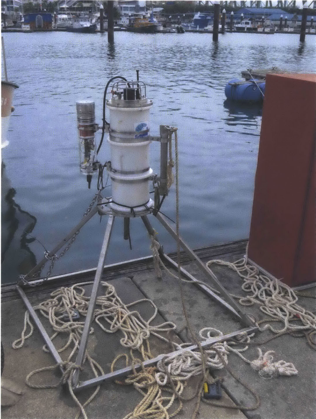
Figure 3-12: PANDA node (white cylinder on tripod) with Optical Modem attached on the left. A black underwater ethernet cable can be seen connecting the two.
