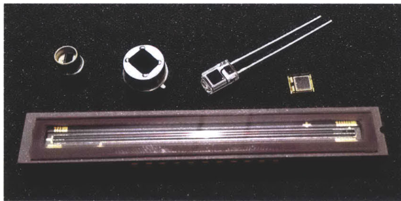
Figure 3-1: Selection of photodetectors. Counterclockwise from the top left, InGaAs photodiode, pyroelectric infrared detector, through hole silicon photodiode, surface mount silicon photodiode, linear CCD array.
