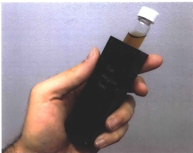
Figure 8-7: Photo of completed hand-held spectrometer. This model discriminates between Diet and Classic Coca-Cola.
