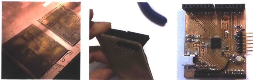
(a) Two Anduinos shortly after milling on the Roland Modela.
