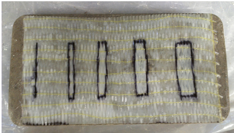
Figure 4-11: FRPP5, FRP-bonded concrete panel Size: Height 7" \times Width 13" \times Depth 4" Multiple crack-like defect sizes: Height 3" \times Widths 0.125", 0.25", 0.5", 0.75", 1" \times Depth 1.5"
