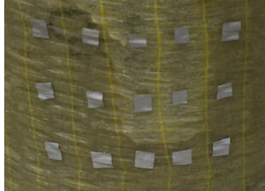
Figure 4-17: Retroreflective tape adhered to specimen
