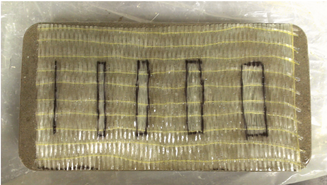
Figure 4-4: Specimen after wet FRP-epoxy layup
