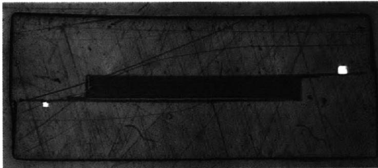
Figure 4-17: Optical microscope image of the cross-section of a 7-layer piezoelectric fiber.
