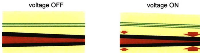
Figure 6-19: Schematic of a modulation mechanism based on a change in angle of incidence.
