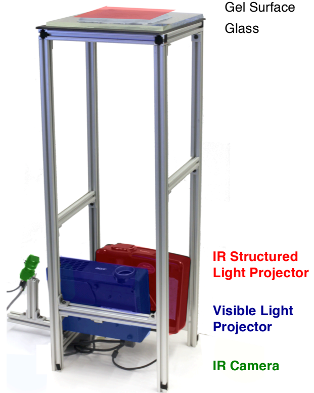
Figure 11. An image of the deForm setup. IR and Visible Light projectors mounted in 80/20 box project upwards through glass to gel surface. An IR camera off to the side captures deformations in the gel.
