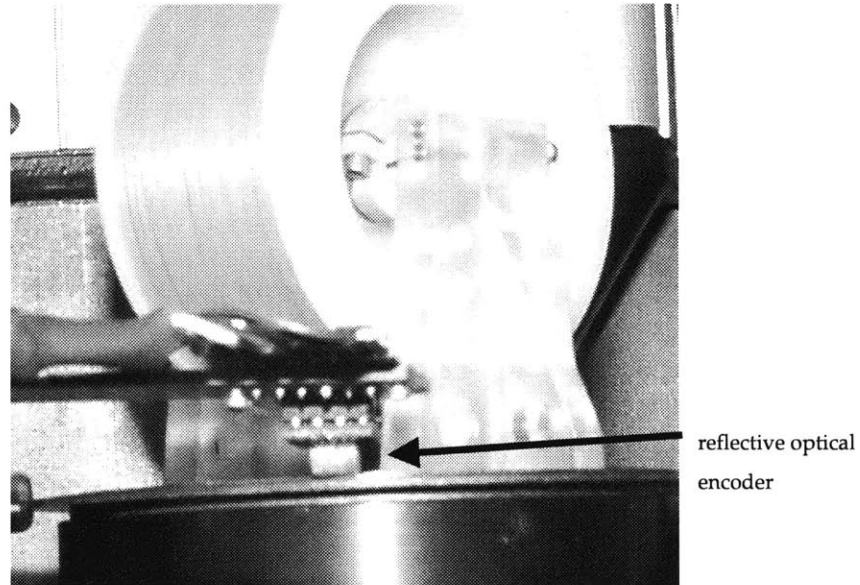
Figure 3.11. Reflective optical encoder mounted on outside edge of untwisting platform.
