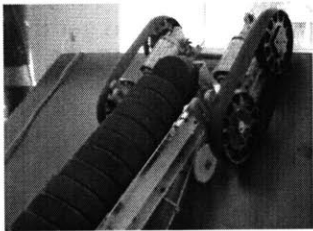
Figure 2.53a Puck Truck mated with Rover and positioned over 5-point hole.
