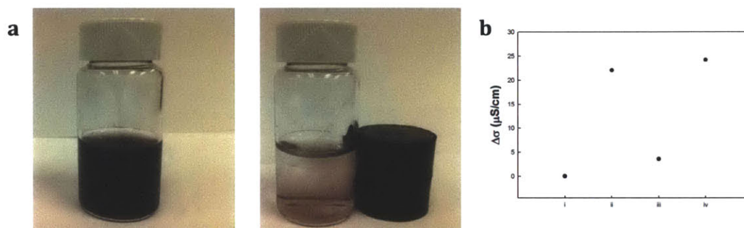
Figure 4.3. (a) The picture that the composite particles can be easily removed by a magnet and (b) the change in conductivity value at each step: (i) the initial value without \text{Cd}^{2+} , (ii) right after adding \text{Cd}^{2+} , (iii) after mixing with the composite particles, followed by that they being removed, and (iv) after the captured \text{Cd}^{2+} being released by heating the solution up to 80\text{ }^\circ\text{C}
