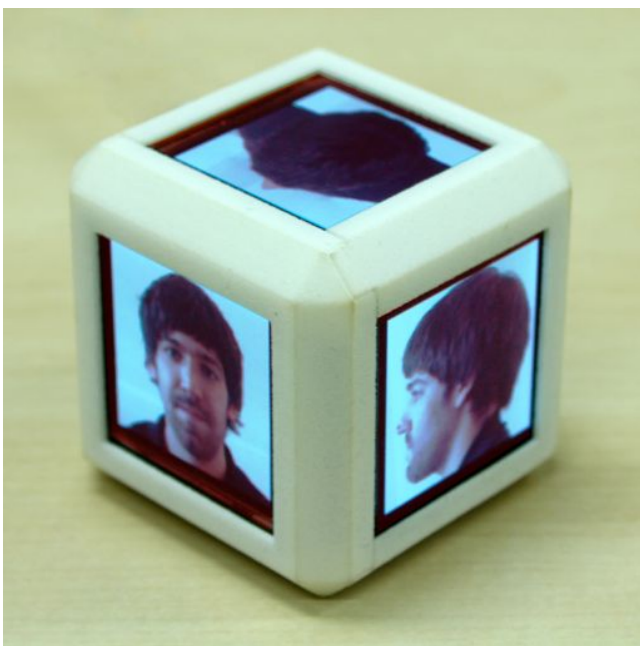
Figure 2. Display Block running the Orthographic Projection application.
