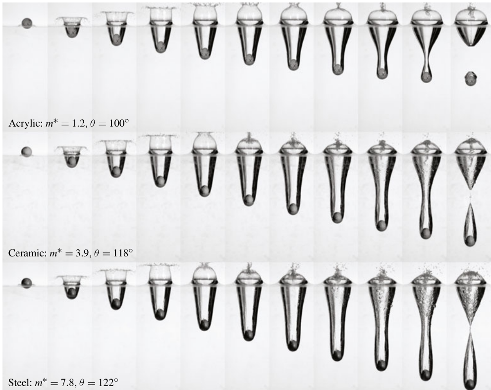
FIGURE 1. Three spheres dropped from the same height ( h = 60 cm), with the same diameter ( D = 2.54 cm), impact speed ( U_0 = 3.43 m s ^{-1} ), and Froude number ( Fr = U_0/\sqrt{gD} = 6.87 ), coated with the same surface treatment to be hydrophobic (note: each sphere takes on a different static wetting angle \theta > 90^\circ due to the nature of the material as indicated for each sequence). The three cases have different mass ratios, m^* = \rho_s/\rho , as indicated. The time between images is 7.1 ms for all cases, and the time to deep seal (cavity pinch-off) is t_{ds} = 70.3, 73.1 and 72.9 ms for the acrylic, ceramic, and steel cases, respectively.
