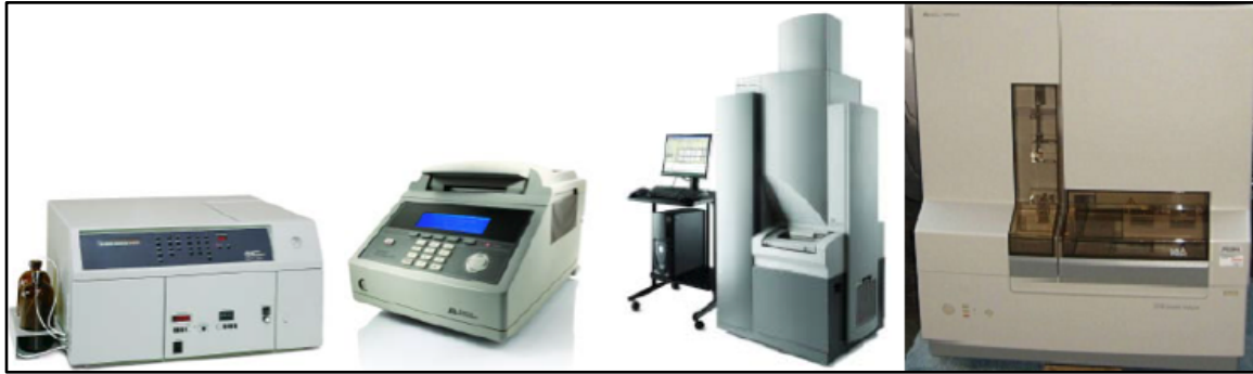
Figure 4: Applied Biosystems DNA synthesizers in 1985, 1997, 2005, and 2011 from left to right (Applied Biosystems, 2013)
