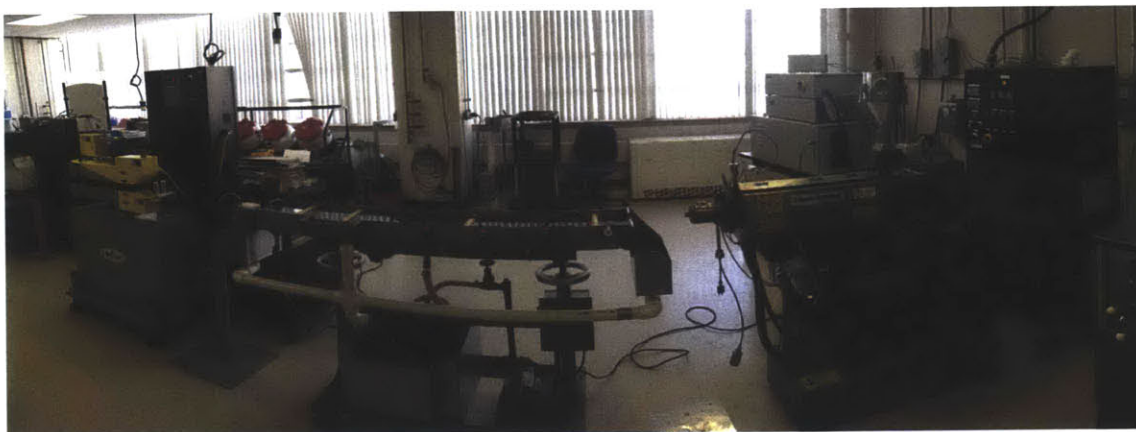
Figure 4: Fiber extrusion assembly at University of Massachusetts - Amherst including single screw extruder, water bath, laser profilometer, and windup unit.
